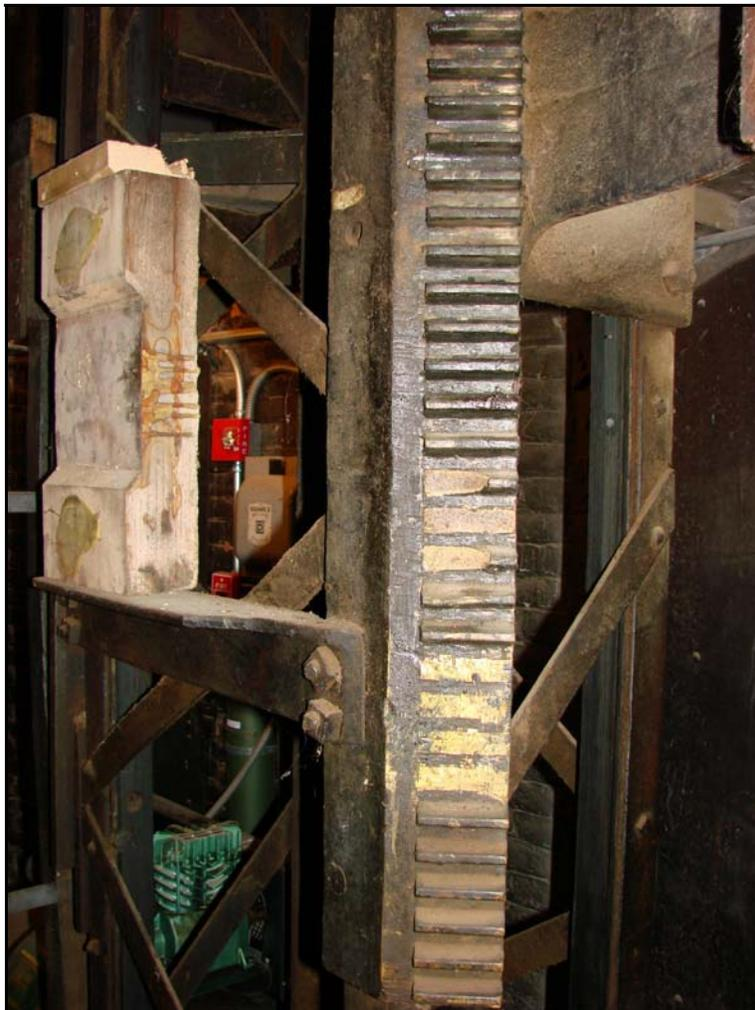
Here on this rack some upper teeth have broken out above the floor leveling section.
